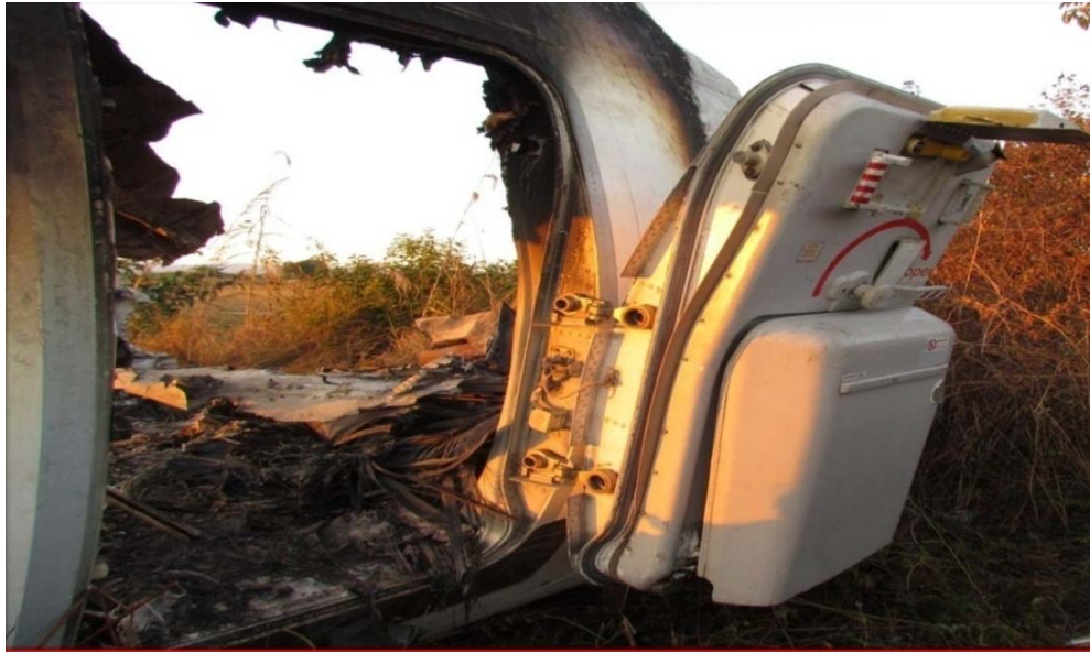
Figure 9 : Forward cabin door (right side)
